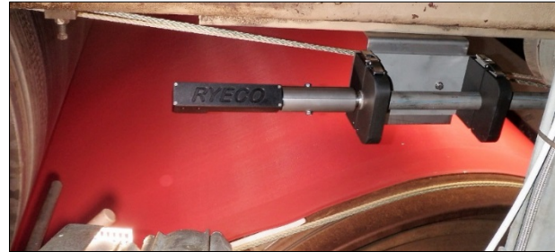
Figure 1: This sensor is installed in on the machine frame parallel to the paper path. This is a paper on felt application. Detection distance is 4 feet (1.2 meters) from the web.
